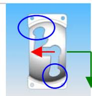
KIP-AIR CON COMANDO PTO ( ← ), DISCESA CON PTO INSERITA ( ↓ ) E NON ( ↘ ) MA SENZA BLOCCO DELLA LEVA SIA IN SALITA CHE IN DISCESA
